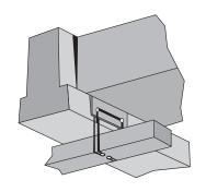
The Ceiling clip is specifically designed to be fixed after beam & block flooring systems have been laid. The Clip is economical and its "knock in" design gives "fix after" flexibility. It allows adjustment for batten size and position and avoids dust, noise and cost of drilling.
