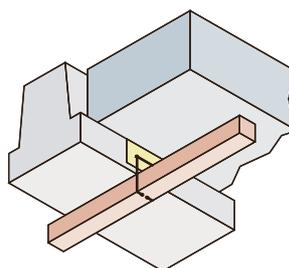
The Ceiling clip is specifically designed to be fixed after beam & block flooring systems have been laid. The Clip is economical and its "knock in" design gives "fix after" flexibility. It allows adjustment for batten size and position and avoids dust, noise and cost of drilling. Available in boxes of 400 from Gordon Products Ltd. Tel:01928 732158
