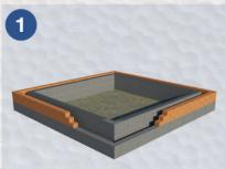
Bearing Wall Construction — The bearing wall is constructed to act as the structural base for the floor. The end walls will need to be erected, equal to or greater than, the top of the beams. This will provide enough friction/anchorage to support the EPS end panel. The damp proof course is rolled into place to prevent the spreading of moisture from the ground.
