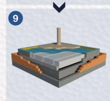
Laying the Concrete Topping The specified structural concrete topping is poured to the required depth, ensuring the EPS infill panels and top sheet are not disturbed during the flow of the concrete. Please note, image is for illustration purposes only and must be carried out by a professional. The concrete shall not be poured on the panels or the load-bearing rails from heights greater than 500mm.
