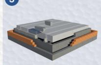
Laying the Closure Blocks — The (optional) concrete closure blocks are designed to correspond with the width of the EPS infill and end panels. A bed of mortar is placed onto the wall between the area where the beams and the blocks are placed, ensuring the top of the block matches that of the beam level. This stage represents the last of the components supplied with the Milbank GDeck solution.
