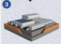
Laying the Infill Panels/Load-bearing Rails – Each wide and narrow panel will come attached with a load-bearing rail. The remaining EPS infill panels are laid between and on top of the concrete beams. Any penetrations, such as plumbing, should be cut circular and tight to the piping, any gaps shall be filled with foam insulation. Install separate load-bearing rails over the multiple beams where required.
