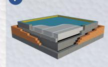
Laying the Perimeter Strips – EPS perimeter strips are installed throughout the screed rail and to any internal walls of the development to eliminate thermal bridging between the walls and the concrete topping.
