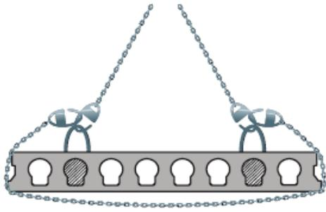
On units over 600mm wide, all 4 lifting devices are used.
