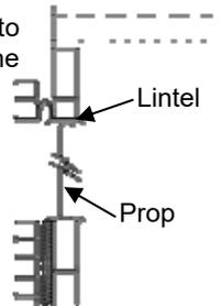
Where the floor units are supported on steelwork, consideration should be given to prevent unequal loading of the steel beams. Propping by the Main Contractor may be required to prevent twisting prior to the floor units being delivered to site.
