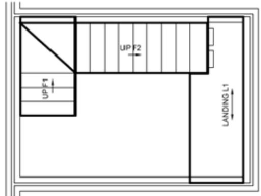
TYPE 7: Storey Height Flight Supported on Side Walls
