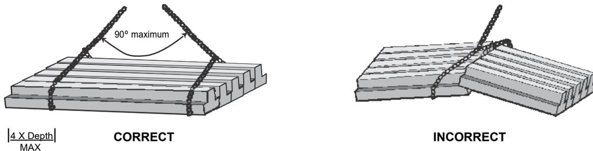
Purpose made block grabs should be used if floor blocks are to be hoisted onto the structures; a safety net should always be attached to the block grabs.
