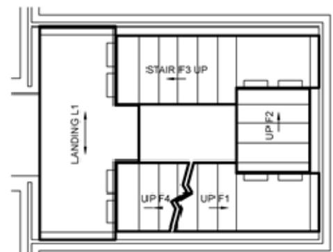
**TYPE 6: Dog Leg Flights with Attached Landings Around a Well**
