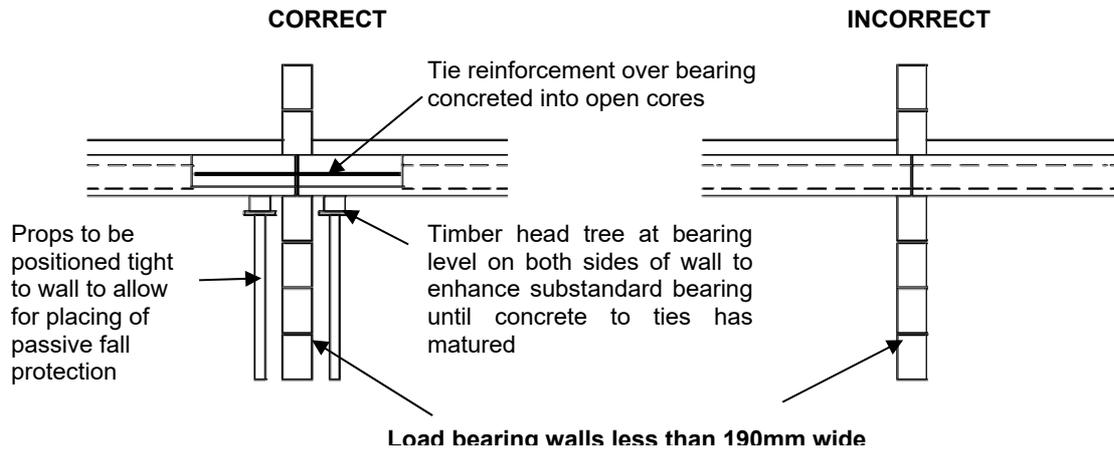
Where units bear onto fair faced walls the Main Contractor must provide protection to minimise the effects of spalling.
